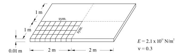
Consider the simply supported rectangular plate above, of thickness  $0.01~\mathrm{m}$  and sides  $4~\mathrm{m}$  and  $2~\mathrm{m}$ , subjected to a uniformly distributed load of  $100~\mathrm{N/m^2}$ .
