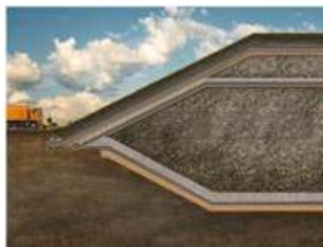
FIGURA 3.7 - Solo Envolvido com Geotêxtil (HUESKER SYNTHETIC GMBH, 2017).
