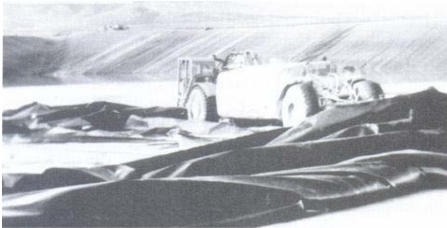
**Figure 3.4 – Example of wind-damaged geomembrane (KOERNER, 1997)**
