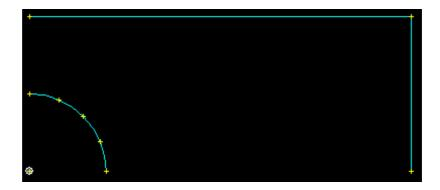
6. Create the geometry for the surface of the plate.
