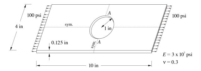
The plate has a circular hole at the center and is submitted to a uniform tension of magnitude 100 psi at two opposite edges. The presence of the hole changes the uniform stress distribution, making the maximum tensile value, which occurs at A, slightly greater than four times the undisturbed value of 100 psi.
