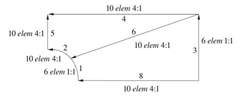
Mesh / Mesh Control / Size Along Curve
