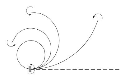
This example uses a simple cantilever beam model to demonstrate the geometric nonlinear effects of large rotations. A linear solution method would not be adequate for this case as equilibrium can only be satisfied in the deformed configuration due to the high applied loading. The example is extensively studied in the literature to demonstrate the efficiency of numerical methods and the large rotation capability of beam, plate and shell elements.
