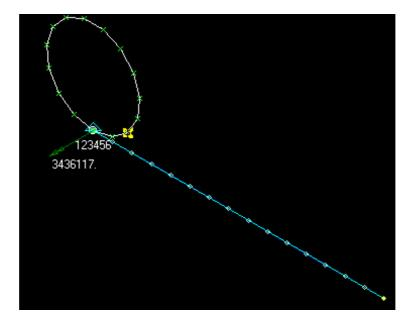
The above shows the actual deformation of the cantilever due to the applied end moment loading.
