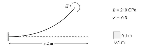
The model consists of a cantilever beam: 3.2 m long, divided into 15 elements, subjected to an end moment of  $\bar{M}=3436117$  N m at the free end, which forces the beam to curl into a complete circle. The beam has a 0.1 m square cross section.
