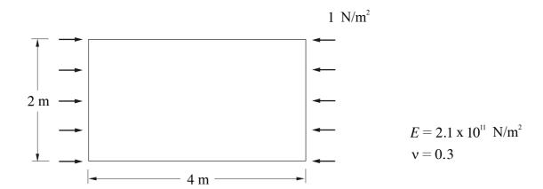
Above is a simply supported rectangular plate, of thickness 0.01 m, subjected to a uniform compressive load of magnitude  $1 \text{ N/m}^2$  on two opposite edges. In linear buckling analysis we solve for the eigenvalues which are scale factors that multiply the applied load (unit in this case) in order to produce the buckling load.
